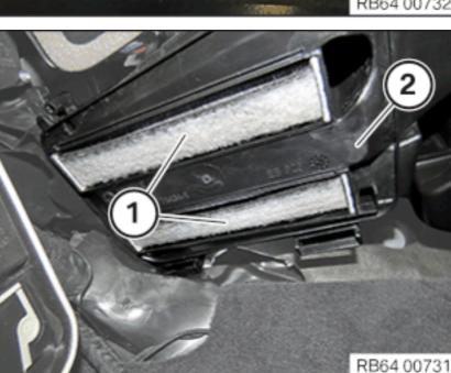
• Slide both microfilters for interior ventilation (1) up into the microfilter housing (2).
