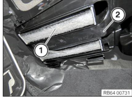
• Remove both microfilters for interior ventilation (1) from the microfilter housing (2) in a downwards direction.
