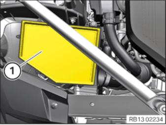
• Feed out air filter insert (1) and remove.
