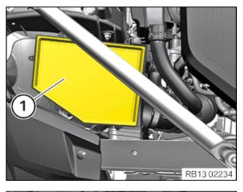
• Install the air filter insert (1).
