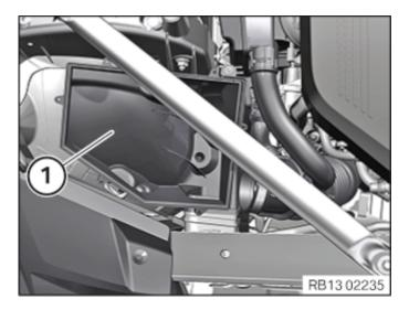
• Clean the lower section of the intake filter housing (1).
