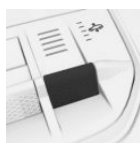
Rocker switch for self-leveling suspension.
