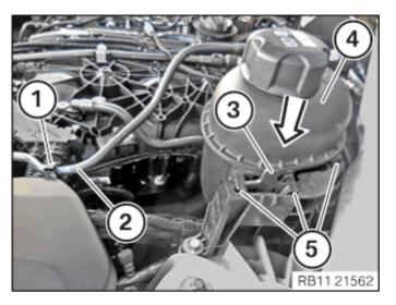
• Feed in the low-temperature coolant expansion tank (4) in **the direction of the arrow** in the guides (5) and install it.
