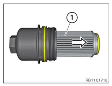
• Release the oil filter element (1) from the oil filter cover in the arrow direction.
