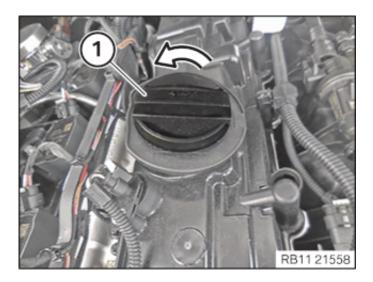
• Open the oil filler cap (1) in the arrow direction.
