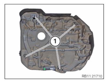
Check the rubber mount (1) for a correct seat of the acoustic cover.
