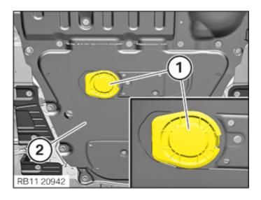
Unlock and open the service flap (1) in the thrust field (2).
