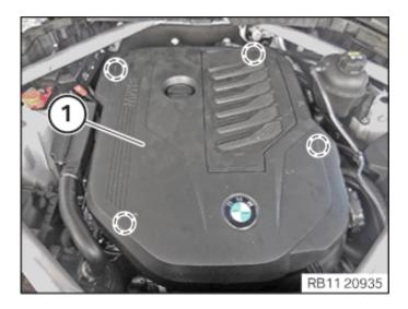
• Install the acoustic cover (1) and fasten it in the rubber mounts (marks).
