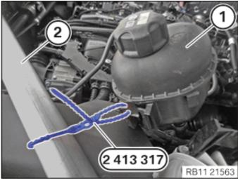
Secure the low-temperature coolant expansion tank(1) with the special tool 2 413 317 on the left front-end strut(2).
