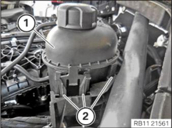
• Position the low-temperature coolant expansion tank (1) **correctly** in the guides (2).
