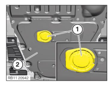
• Close and lock the service flaps (1) in the thrust field (2).
