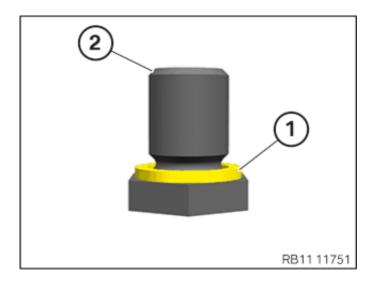
• Renew the sealing ring (1) at the oil drain plug (2).
