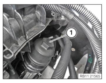
• Release the oil filter cover (1) with standard tools.
