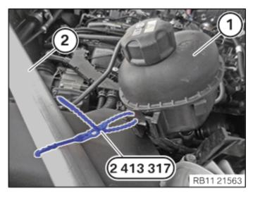
Feed out and remove special tool 2 413 317 between the front-end strut (2) and the lowtemperature coolant expansion tank (1).
