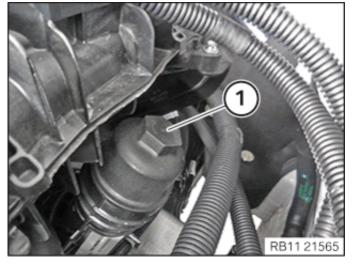
• Tighten the oil filter cover (1).
