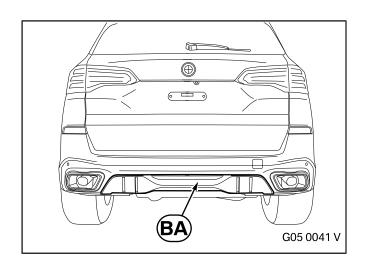
Remove standard rear diffuser as described in **ISTA/AIR**.
