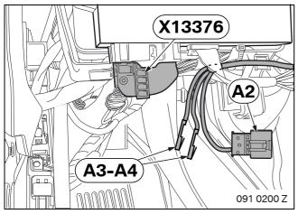
Separate socket contacts from branches **A3** and **A4** and connect with a miniature connector to plug **X13376** (41 pin SW):
