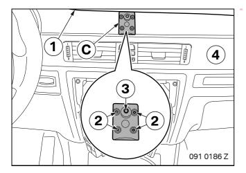
Hold base plate **C** centrally over the hazard lights switch and flush with the top edge (1).
