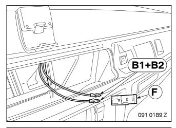
Connect branches **B1** and **B2** to socket casing **F** (GN 2-pin), as follows:
