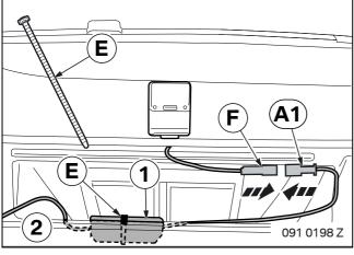
Connect socket casing **F** to branch **A1**.
