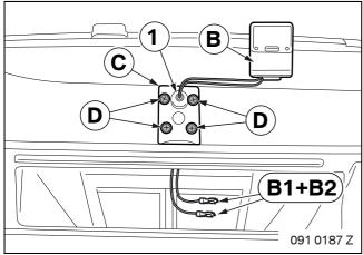
Secure base plate **C** using Philips screws **D**.
