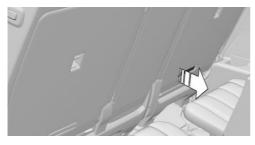
Pull the loop and fold the rear seat backrest forward.
