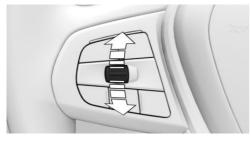
Press the rocker switch up or down repeatedly until the desired speed limit is set.
