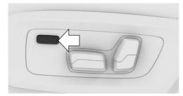
Press the button to reset to standard position. The process is canceled if the button is pressed again.
