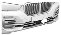
The radar sensor is located in the front bumper. Always keep radar sensor clean and unobstructed.
