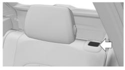
Pull the lever and fold the rear seat backrest forward.
