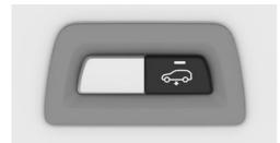
When the tailgate is opened, the vehicle can be lowered to the entry level and raised again by pressing the button. The flashing of the LED in the button indicates the level change.
