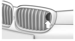
The camera is automatically heated when the external temperatures are low. When the vehicle lighting is switched on, the camera objective is cleaned at regular intervals when the windshield washer system, refer to page 141, is activated.
