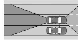
Four radar sensors in the bumpers monitor the space next to the vehicle from a minimum speed of up to approx. 130 mph/210 km/h.
