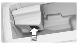
3. Remove the cover of the fragrance cartridge. Hold the cover on the top to slide it from the fragrance cartridge.
