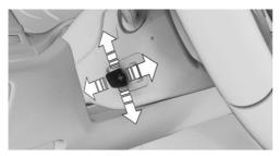
Move the steering wheel to the preferred height and angle to suit your seating position by pressing the switch.
