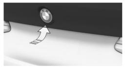
Without Comfort Access: unlock the vehicle, then press the button on the outside of the tailgate. With Comfort Access: unlock the vehicle or carry the remote control with you and then press the button on the outside of the tailgate.
