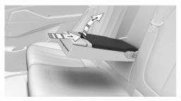
Press the button, arrow 1, and fold the cover up, arrow 2.
