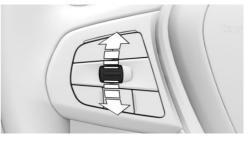
Press the rocker switch up or down repeatedly until the desired speed is set.
