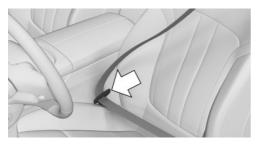
To ease accessibility to the safety belt buckle, an adjustable slider is available on the belt to help position the buckle when not in use.
