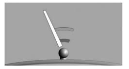
Two static circle segments show the distance between the trailer and the trailer hitch.
