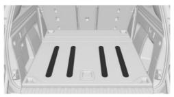
The system prevents slipping of the cargo in the cargo area.
