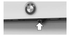
The camera lens is located in the handle of the tailgate.
