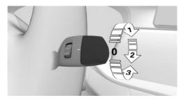
Turn the outer switch upward.
