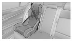
The safety belts in the rear and the front passenger safety belt can be permanently locked to fasten child restraint systems.
