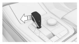
Activate the sport program/manual mode: Press the selector lever to the left out of selector lever position D.
