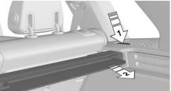
Press the release button, arrow 1, and pull the cargo cover out toward the rear, arrow 2.
