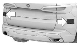
The radar sensors are located in the rear bumper.
