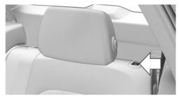
Pull the switch. The rear seat backrest folds forward.
