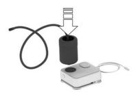
4. Screw the filling hose of the sealant container onto the tire valve of the nonworking wheel.
