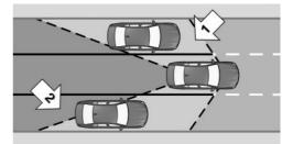
Two radar sensors in the rear bumper monitor the area behind and next to the vehicle when traveling faster than a minimum speed.
