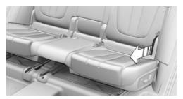
Pull the loop and fold the rear seat backrest forward.
