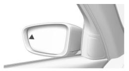
The light in the exterior mirror flashes if vehicles are detected by the rear sensors and your own vehicle is moving backwards.
