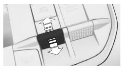
Push the rocker switch forward or pull it back repeatedly until the desired xOffroad driving mode is displayed in the instrument cluster.
