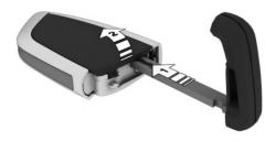
3. Push battery in the direction of the arrow using a pointed object and lift it out.
