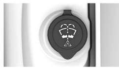
The washer fluid reservoir is located in the engine compartment.
