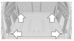
There are four lashing eyes in the cargo area for securing cargo.
