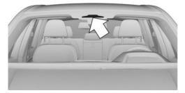
The camera is installed near the interior mirror. Keep the windshield in front of the interior mirror clean and clear.
