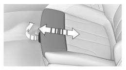
Pull the lever at the front of the seat and push the thigh support forward or back.
