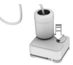
Let the compressor run for max. 10 minutes to fill the tire with sealant and achieve a tire inflation pressure of approx. 2.0 bar.
