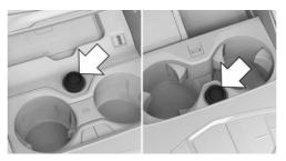
A socket is located between the cup holders in one of the marked positions.
