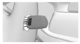
Turn the thumbwheel on the wiper lever.
