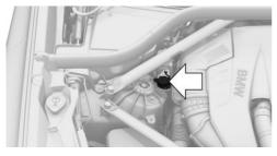
The starting aid terminal in the engine compartment acts as the battery's positive terminal. Open the cover of the starting aid terminal.
