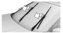
3. Press the button, arrow 1, and pull out the wiper blade, arrow 2.
