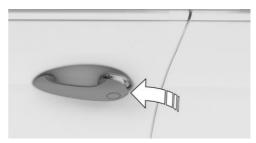
Guide one finger of your other hand from the back under the cover and push the cover out. Use the thumb for counter support to prevent the cover from falling out of the door handle.
