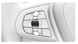
Press the rocker switch up or down once while the system is interrupted. The system will be activated.
