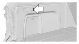
The buttons of the cargo cover are located in the cargo area.
