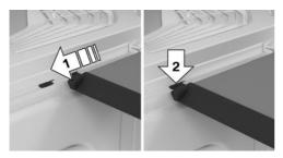
To restore the functionality, close the cargo cover by hand, arrow 1, until it engages in the mounting, arrow 2.
